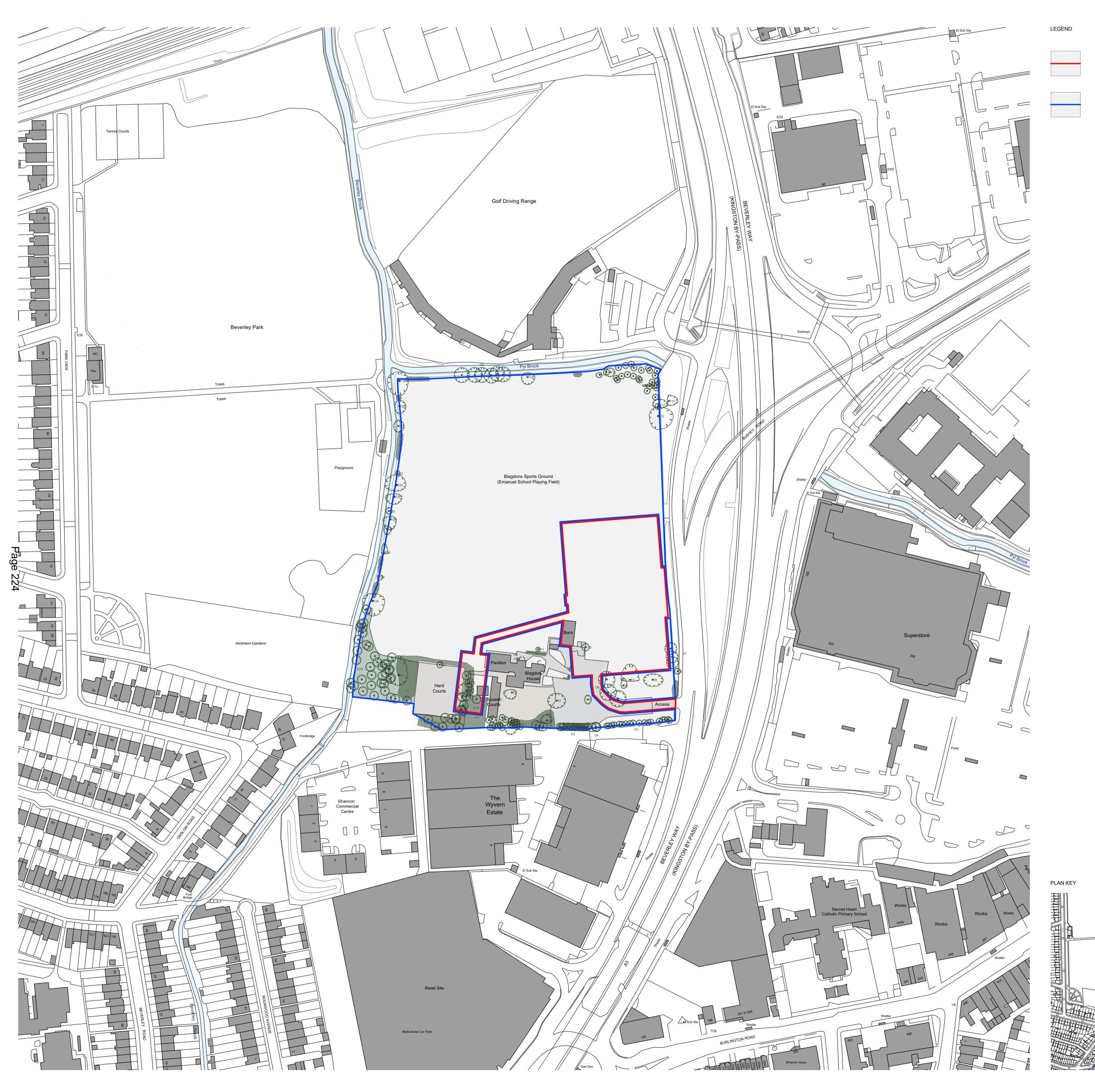
APPLICATION SITE AREA (8000M2) REQUIRED FOR PROJECT CONSTRUCTION PHASE WITH ACCESS ADJOINING BEVERLEY WAY
